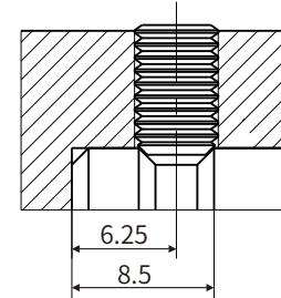
Use M5 internal hexagon flat-end setting screws for fixation with a maximum torque of 0.5 N/m
