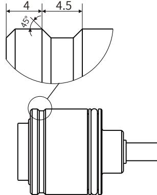
Flange shell with O-ring and auxiliary washer
