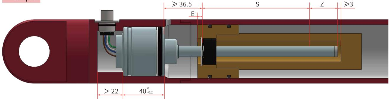
The assembly method depends entirely on the design of the hydraulic cylinder. The commonly used assembly method is to install from the rod end of the hydraulic cylinder, or to install from the cylinder head end of the hydraulic cylinder. In both assembly methods, O-ring and auxiliary gasket are used for air sealing.
